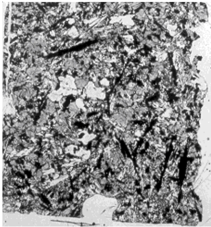
Figure 3a, b: Thin section photos showing abundant, platy ilmenite in 71055.
