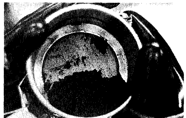
→ FIGURE 4-33. — Soil retained on sieve 140 (0.105 mm) from core-tube-2 sample. (LRL photograph S-69-45107)
