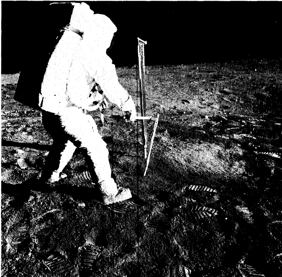
FIGURE 1-34.— The astronaut is collecting a core-tube sample for later study by scientists. The SWC experiment is still deployed. (NASA AS11-40-5964)
