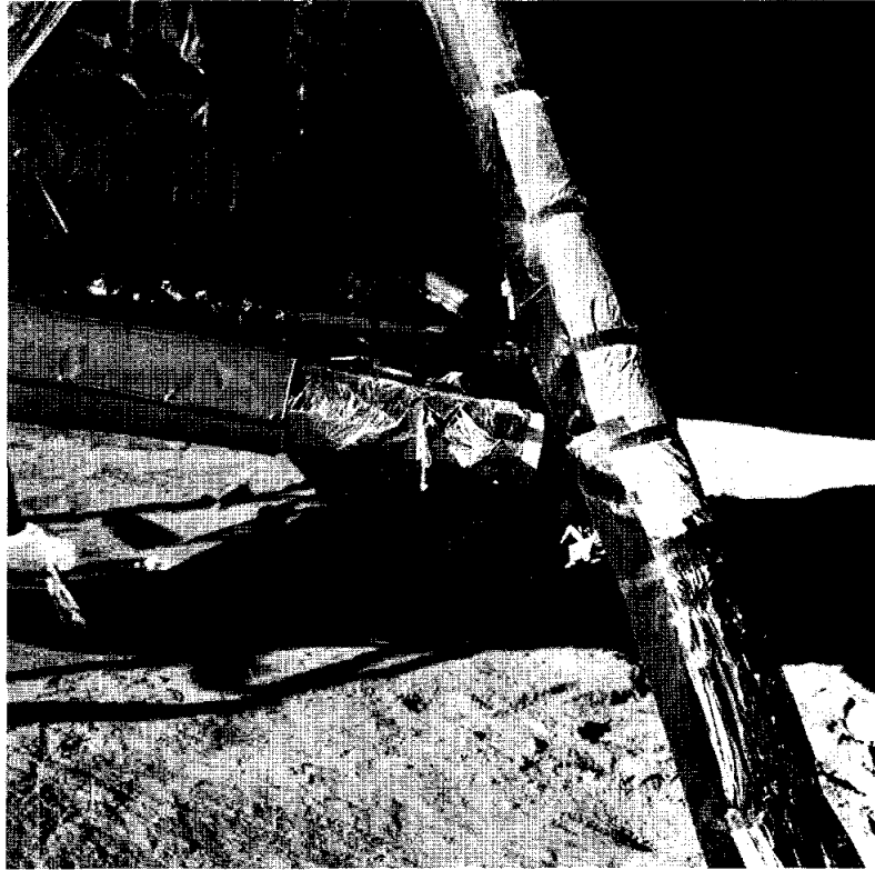
FIGURE 4-18.—Primary strut and secondary strut of the +Y footpad after touchdown. (NASA AS11-40-5919)
