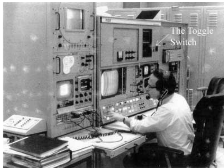
Figure 6 The Honeysuckle Creek RCA scan-converter. Ed von Renouard is at the desk. The toggle switch can be seen directly above his head (Photo: Hamish Lindsay).
